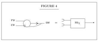
It should be noted that this  $\underline{ml}$  corresponds to the actual vacuum tube trigger circuits mentioned at the beginning of 5.1. It is worth mentioning that  $\underline{ml}$  contains one E-element, while the simplest trigger circuits contain one or two vacuum tubes (cf. loc. cit.), in agreement with the estimates of 6.5.
