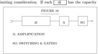
dlis to be used as a memory its output must be fed back—directly or indirectly—into its input. In an aggregate of many dl organs—which M is going to be—we have a choice to feed each back into itself, or to have longer cycles of dl 's: Figure 19 (a) and (b), respectively. dl
