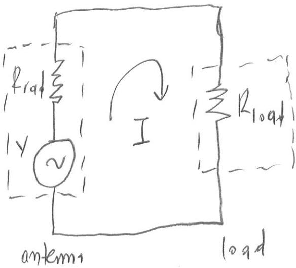
The sketch shows the effective circuit of an antenna used as a receiver. The radiation induces a voltage  $V$  across the antenna terminals, which appears to the load as an ideal generator in series with the antenna's radiation resistance.
