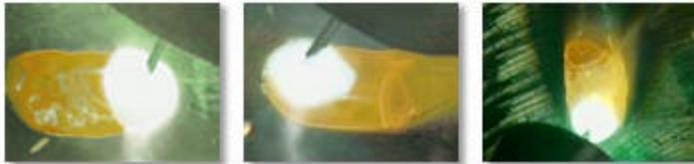
MIG welds tend to be clean, although with some splatter, and because of the lack of oxidation one can weld several times over the same spot. The drawback is that one cedes the parameter of amount of new material to the machine.
