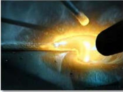
Here, two pieces of metal are being joined. A small gap between them allows for complete heating, while a third piece of metal (welding rod, or copper clad) is brought in to ensure that the final weld is as thick or thicker as the original material. In addition, the copper on the copper clad rod acts as a flux (similar to the rosin in solder) to help smooth the process.
