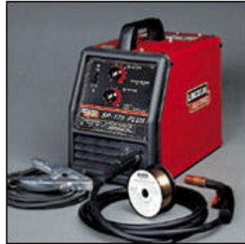
Metal/Inert Gas welding uses a wire, electricity, and gas to produce clean, fast, repeatable joins. An inert gas surrounds the arc and shields it from the atmosphere to prevent oxidation. Argon, Nitrogen, and “Tri Gas” are commonly used, depending on metal and application. MIG can weld aluminum as well as steel.
