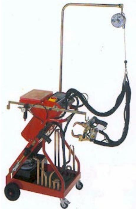
Spot welding is used when full joins are not necessary, and especially on plate and sheet metal, where the warping caused by other welding techniques would be unacceptable. Most metal chassis are spot welded. Two electrodes, typically copper, are placed outside two directly abutted pieces of sheet. Electricity passes through the electrodes to the sheet, where the resistance of the metal leads to heat, causing melting and joining.
