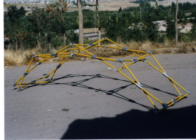
Figure 16: Barrel vault foldable structure
