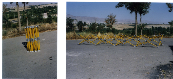
Figure 15: Flat foldable structure in the folded and fully deployed configurations
