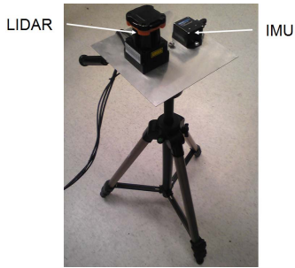
Fig. 5. Nodding device for collection of LIDAR data.
