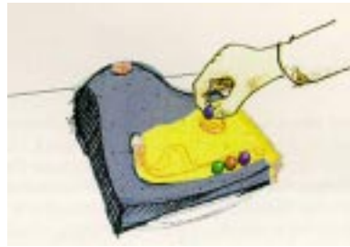
Figure 3.4 Messages can be played back by placing their marble on a small indentation on the machine.
