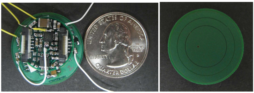
Fig. 2. Photograph of assembled circuit. (Left). The top side of the two-board structure with components. (Right). The bottom side of the bottom PCB. The metal plate on the bottom is the sensing element, which is covered by solder mask.
