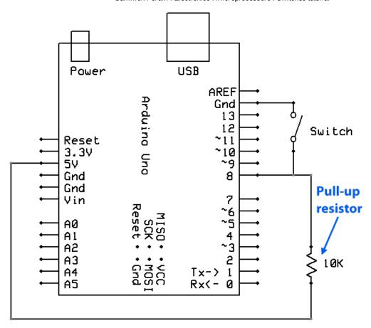
This resistor "weakly" pulls the switch up to +5V, so that if the switch is open, it will have 5V on it (through the resistor) and thus will register HIGH if not pressed, and LOW if pressed.
