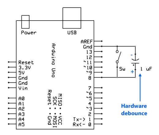
In this case the capacitor is charged by the pull-up resistor. When the switch is pressed it discharges, and takes a moment to charge again. This delay effectively debounces the switch, so the simpler code above (without the debounce) could be used.
