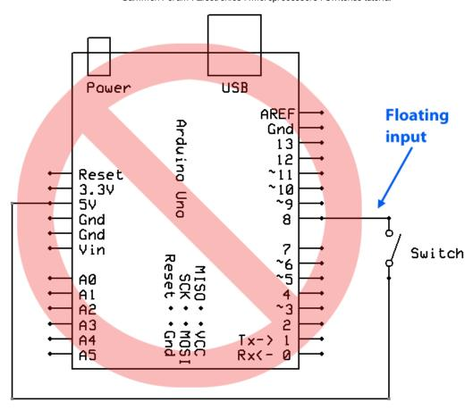
This will not work properly because the switch input (digital pin 8 in this example) is "floating" if the switch is open.
