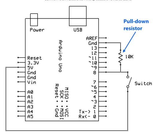
This resistor "weakly" pulls the switch down to ground, so that if the switch is open, it will have oV on it (through the resistor) and thus will register LOW if not pressed, and HIGH if pressed.
