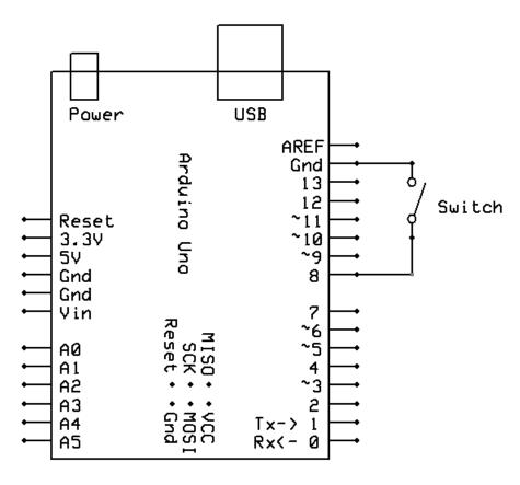
This internal pull-up "weakly" pulls the switch up to +5V, so that if the switch is open, it will have 5V on it (through the resistor) and thus will register HIGH if not pressed, and LOW if pressed.
