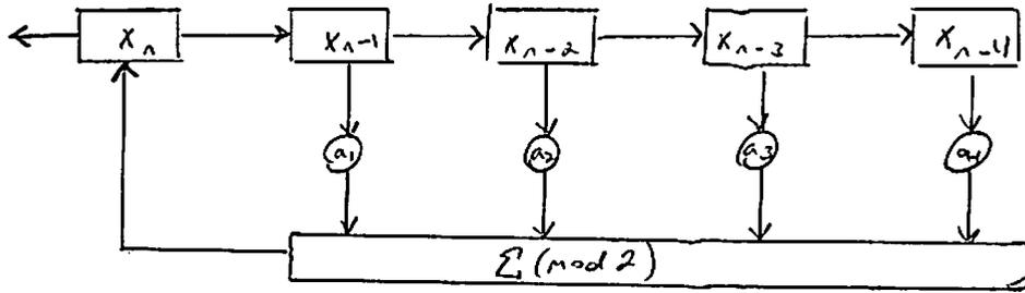
Maximal taps for 4<sup>th</sup> order use  $X_n = X_{n-1} + X_{n-4}$  (from table 6.1)
