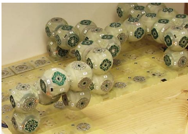
Fig. 1 Two Soldercubes assemblies consisting of a total of 27 Soldercube modules. Modules are located on an a tiled experiment substrate. The smaller assembly on the left is used to demonstrate locomotion in Sect. 4.4, pictured here while performing a step spanning two substrate tiles. The larger assembly on the right is a four-legged robot used to demonstrate synchronized motion between eight modules in Sect. 4.5
