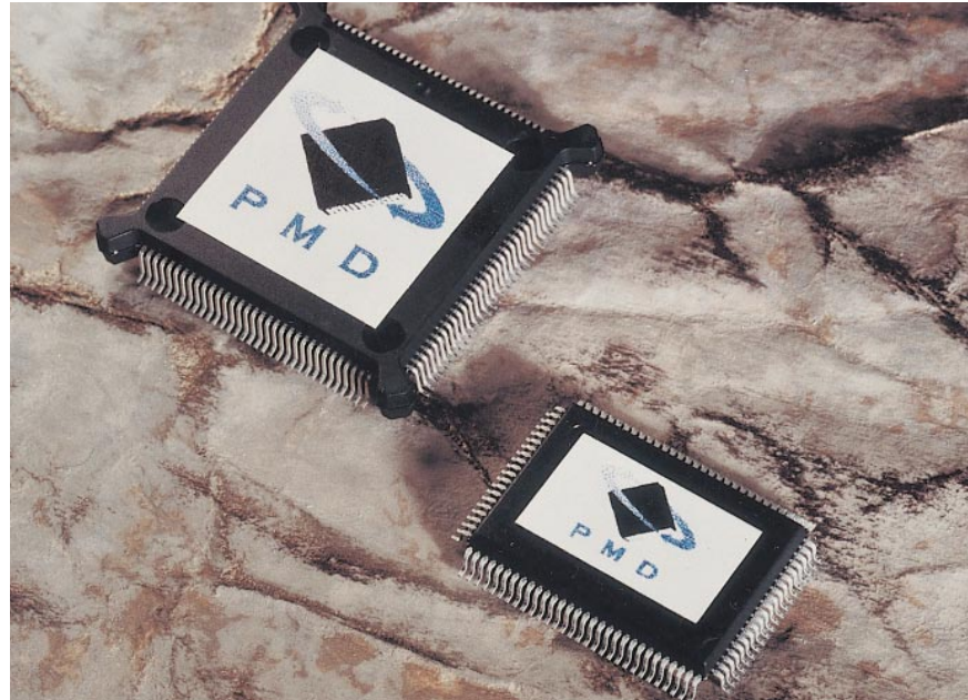
A motion processor is an integrated circuit geared for motion control. Some are single-chip, others, as in the case of the Navigator MC2100 processor for brushed servo motors, consist of several chips.
