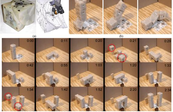
INTERNAL ROTATION & MAGNETIC CONECTION
