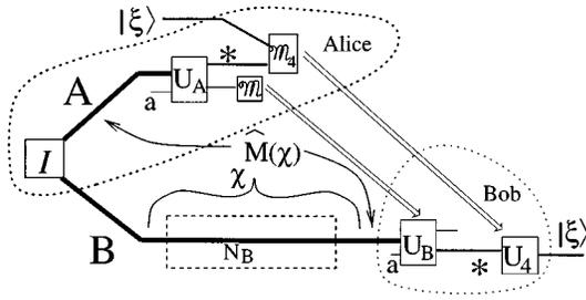
FIG. 15. A 1-EPP can be transformed into a QECC. Given  $\chi$ , Alice creates mixed states  $\hat{M}(\chi)$  by passing halves of entangled states  $\Phi^+$  from source  $I$  through the channel. Alice and Bob perform a 1-EPP resulting in perfectly entangled states (\*) which are then used to teleport  $|\xi\rangle$  safely to Bob, completing a QECC.
