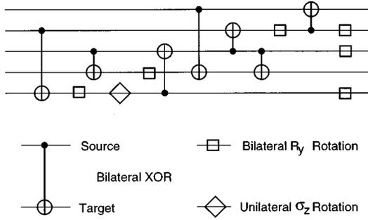
FIG. 18. The quantum gate array, determined by our computer search, which protects one qubit from single-bit errors in a block of five. “Bilateral” and “unilateral” refer to whether both Alice and Bob, or only Alice (or Bob), perform the indicated steps in the 2-EPP; in the QECC version, it corresponds to whether the operation is done in both coding and decoding, or in just the coding (or decoding) operations. All but the first qubit are measured at the end.
