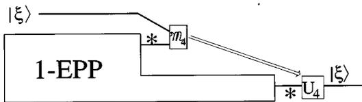
FIG. 4. If the 1-EPP of Fig. 3 is used as a module for creating time-separated EPR pairs (\*), then by using quantum teleportation [5], an arbitrary quantum state  $|\xi\rangle$  may be recovered exactly after  $U_4$ , despite the presence of intervening noise. This is the desired effect of a quantum error-correcting code (QECC).
