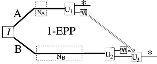
FIG. 3. One-way entanglement purification protocol (1-EPP). In 1-EPP there is only one stage; after unitary transformation  $U_1$  and measurement  $\mathcal{M}$ , Alice sends her classical result to Bob, who uses it in combination with his measurement result to control a final transformation  $U_3$ . The unidirectionality of communication allows the final, maximally entangled state (\*) to be separated both in space and in time.
