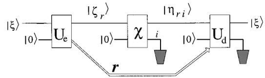
FIG. 13. A general one-way QECC. A classical side channel from Alice to Bob is allowed in addition to quantum channel  $\chi$ .
