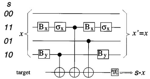
FIG. 11. Step  $k$  of the one-way breeding protocol. The scheme is very similar to the hashing protocol of Fig. 10, except that the target for the BXOR's is guaranteed to be a perfect  $\Phi^+$  state. This allows the one-bit operations to be undone so that there is no back-action on the string  $x$ .
