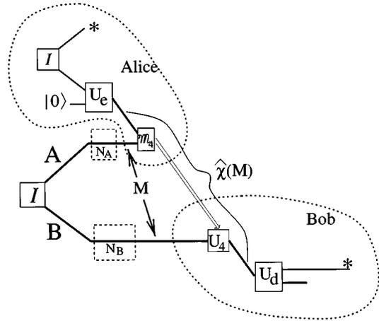
FIG. 14. A QECC can be transformed into a 1-EPP. Teleporting  $(M_A, U_d)$  via a mixed state  $M$  defines the noisy channel  $\hat{\chi}(M)$ . If a quantum error-correcting code  $\{U_e, U_d\}$  can correct the errors in this channel, the code and channel can be used to share pure entanglement between Alice and Bob (\*). This establishes inequality (52), viz.,  $\forall_M D_1(M) \geq Q(\hat{\chi}(M))$ .
