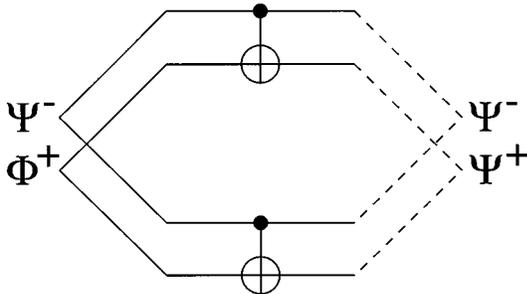
FIG. 6. The BXOR operation. A solid dot indicates the source bit of an XOR operation [32] and a crossed circle indicates the target. In this example a  $\Psi^-$  state is the source and a  $\Phi^+$  is the target. If the pairs are later brought back together and measured in the Bell basis the source will remain a  $\Psi^-$  and the target will have become a  $\Psi^+$ , as per Table I.
