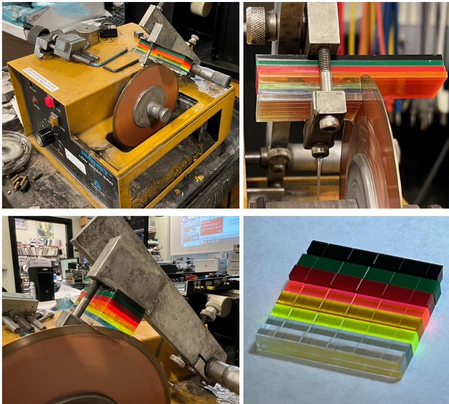
Figure 4: Process to cut thin cross sections of the minimally laser-cut acrylic samples.
