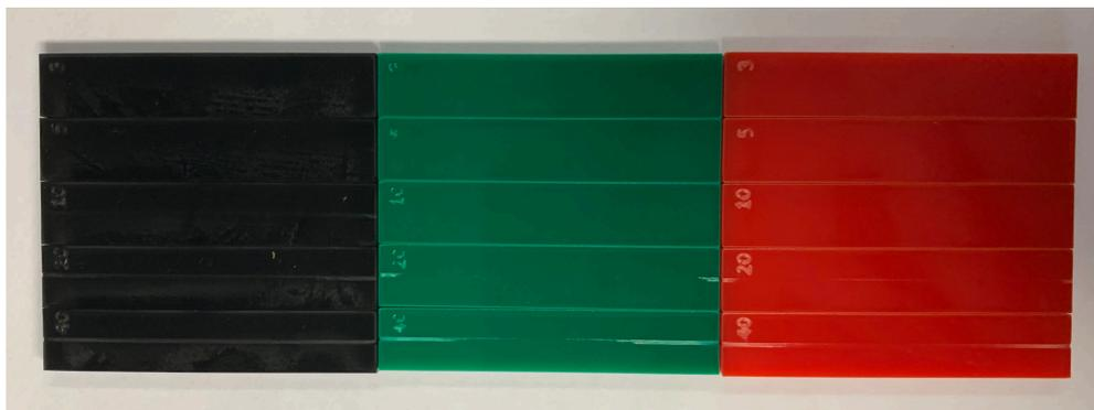
Figure 10: Minimally laser-cut opaque (black, green, red) acrylic samples on the XTool S1 (455 nm) 40 W blue diode laser at 300 mm/s with a power percentage of 40, 20, 10, 5, and 3, respectively.
