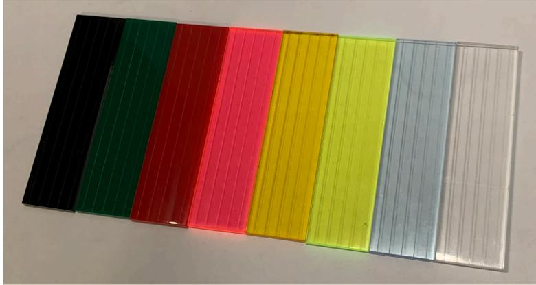
Figure 3: Minimally laser-cut opaque (black, green, red) and transparent (pink, orange, yellow, blue, clear) acrylic samples on the 10,640 nm CO<sub>2</sub> laser.
