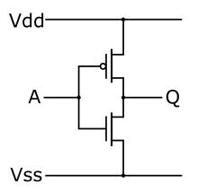
This is a plain inverter, the text says to add a control input to it that can force the output to a disconnected state. So I guess this is a two inputs to three outputs kind of thing, where our outputs are HIGH, LOW, and DISCONNECT. Lol.
