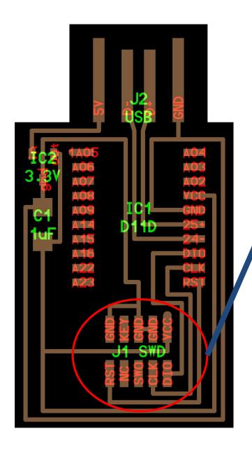
Programming header—how you (initially) load code onto this microcontroller!
