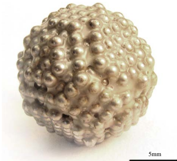
Figure 13 An 832 voxel sphere made of 1.5 mm steel spherical voxels and infiltrated with polyvinyl acetate glue
