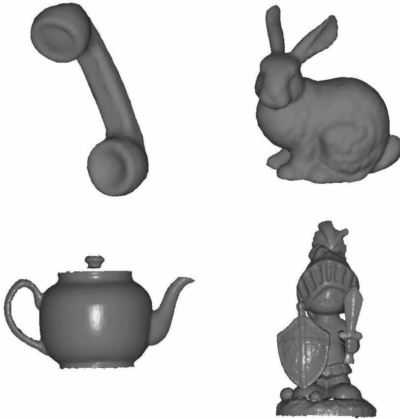
Figure 7: Marching Triangle Reconstruction of 3D Models for Real Objects
