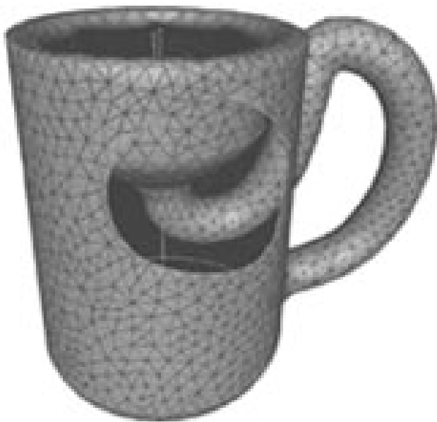
Figure 7: A Klein mug. A single, self-intersecting surface whose handle and outside and inside walls are each controlled by cylinder tools (800 nodes).
