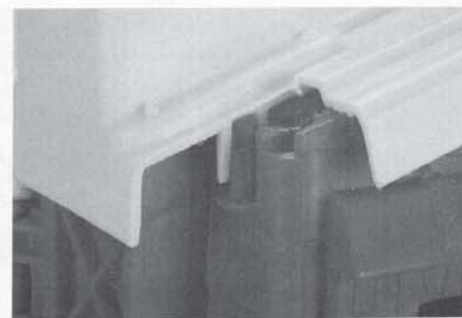
FIGURE 4.18 Another type of annular snap uses molded-in serrations to create a pine tree-like shape that aids in interlocking in an annulus simply from compression forces from elastic spring-back and from friction. (Photograph courtesy of Fisher-Price, East Aurora, NY; used with permission.)
