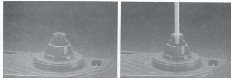
FIGURE 4.17 Photograph showing the use of an annular snap-fit in a child's toy. The cut-away annulus (left) is elastically deflected by the relatively more rigid post to allow engagement and locking (right). (Photograph courtesy of Fisher-Price, East Aurora, NY; used with permission.)
