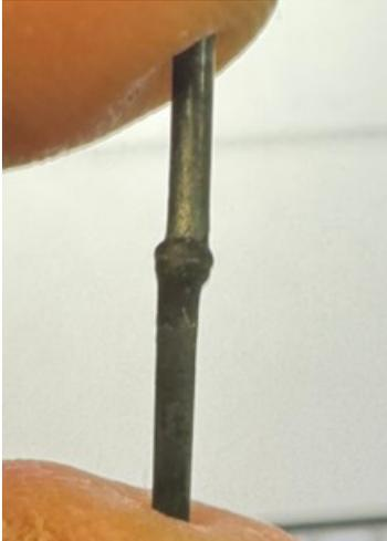
The samples produced show excellent bonding and mechanical properties. One of the more interesting features of this process is the ability to weld non line of sight materials which is not a feature available to most welding modalities like laser, e-beam, TIG, MIG, etc. This differs from resistance welding in that you do not melt the part, and you operate in a completely different voltage and power regime.
