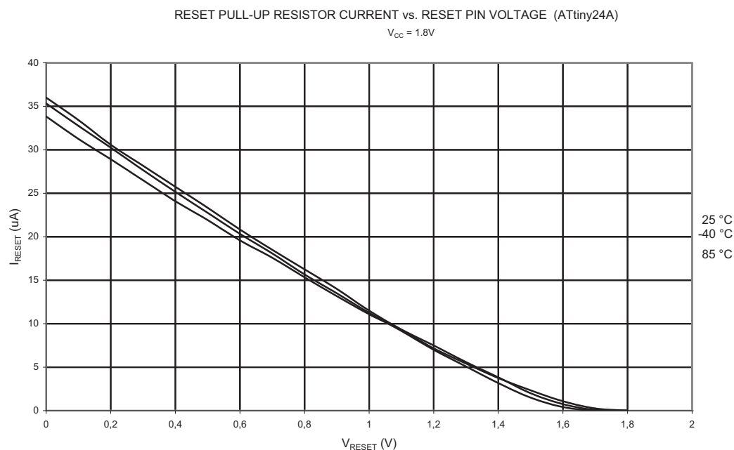
Figure 21-24. Reset Pull-up Resistor Current vs. Reset Pin Voltage ( V_{CC} = 1.8V )
