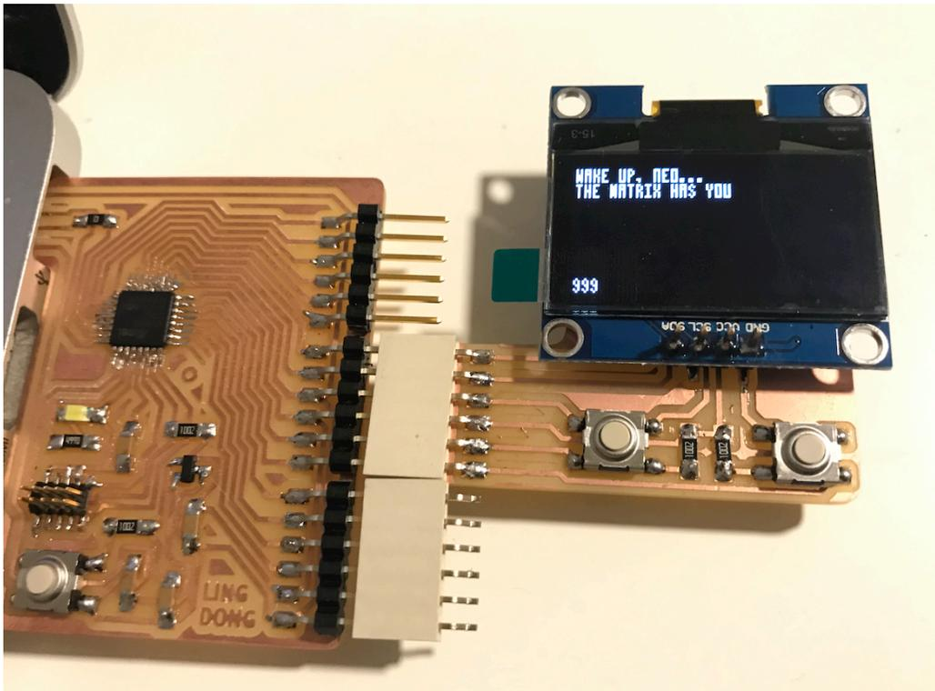
It includes options to use software/hardware I2C, and which I2C pins to use; just fiddle with the macros on the top of the file.
