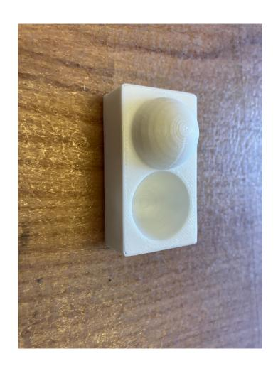
With default surface finish settings, we clearly can see the layers. Further optimization is necessary for smoothing the surface finish.
