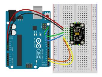
Board 5V to sensor Vin Board GND to sensor GND Board SCL to sensor SCL Board SDA to sensor SDA Board 2 to sensor GPIO Board 3 to sensor XSHUT
