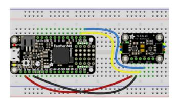
Board 3V to sensor VIN (red wire)
