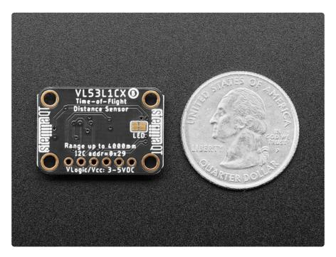
This is the 'next generation' of the <u>VL53L0X ToF sensor</u> (http://adafru.it/3317) and can handle about "30 to 4000mm of range distance, with up to 50Hz update rate. If you need an even smaller/closer range, check out the <u>VL6180X</u> (http://adafru.it/3316) which can measure 5mm to 200mm and also contains a light sensor.
