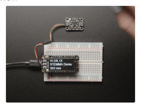
The Adafruit VL53L1X Time of Flight Distance Sensor (also known as VL53L1CX) is a Time of Flight distance sensor that has a massive 4 meter range and LIDAR-like precision. The sensor contains a very tiny invisible laser source and a matching sensor. The VL53L1X can detect the "time of flight", or how long the light has taken to bounce back to the sensor.
