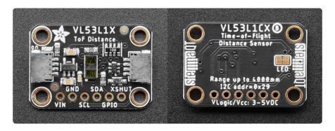
This breakout ships with a protector over the sensor. It must be removed before use! See details at the bottom of the Overview page.
