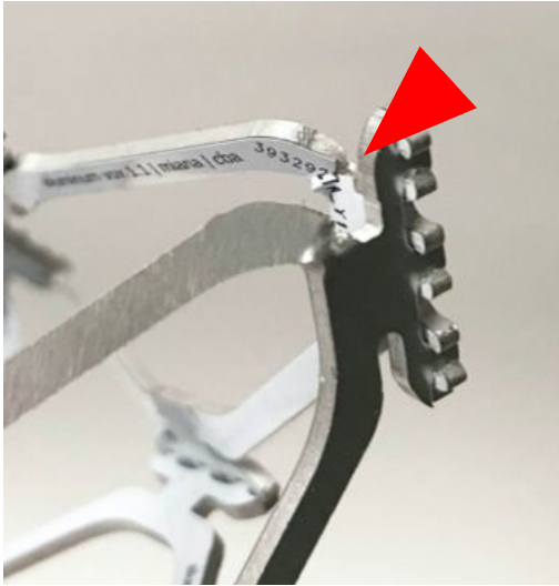
Aluminum cuboct voxel failure at 50% strain
