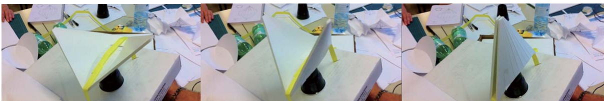
Fig 12: Stage 2. Group Brief: Dynamic Solar Shading (members: Emilie Hergott, Nicolas, Leduc, Sophie Pennetier, and Simon Schleicher); upward motion actuated by downward force on exterior edge
