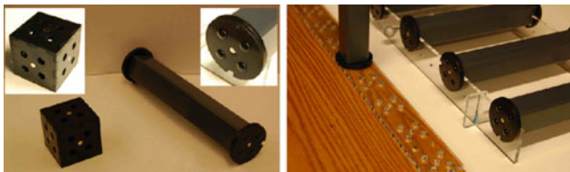
(a) A node (left) and a member (right) (b) Part bins containing parts with close up views
