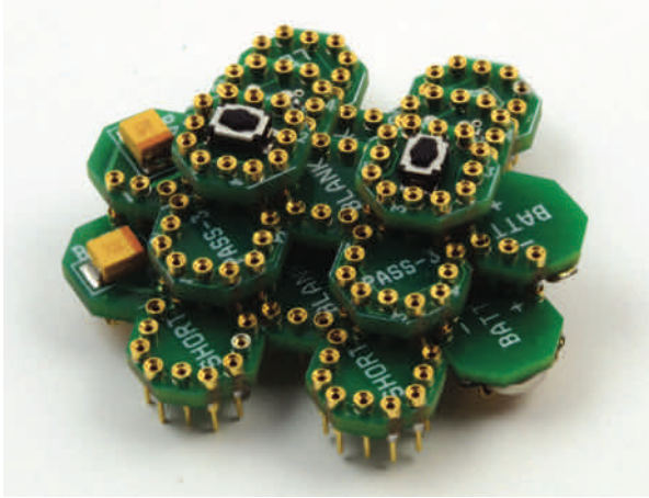
Fig. 14. Two channels (play and stop) of an infrared remote control printed with the Bitblox printer.
