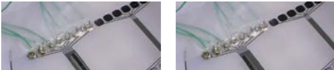
Figure 2-12: Demonstration of electrostatic actuation of a 1 mm aluminum tube, showing proof of concept for the Electrostatic Catoms. (Karagozler [50])
