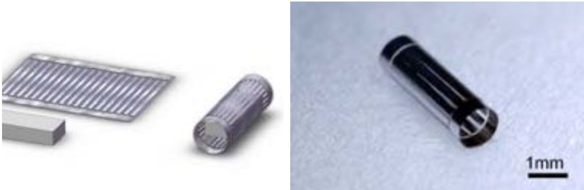
Figure 2-10: Microfabrication process for aluminum-on-silicon-dioxide tubes to be used for the electrode shells of electrostatic Catoms. (Karagozler [50])
