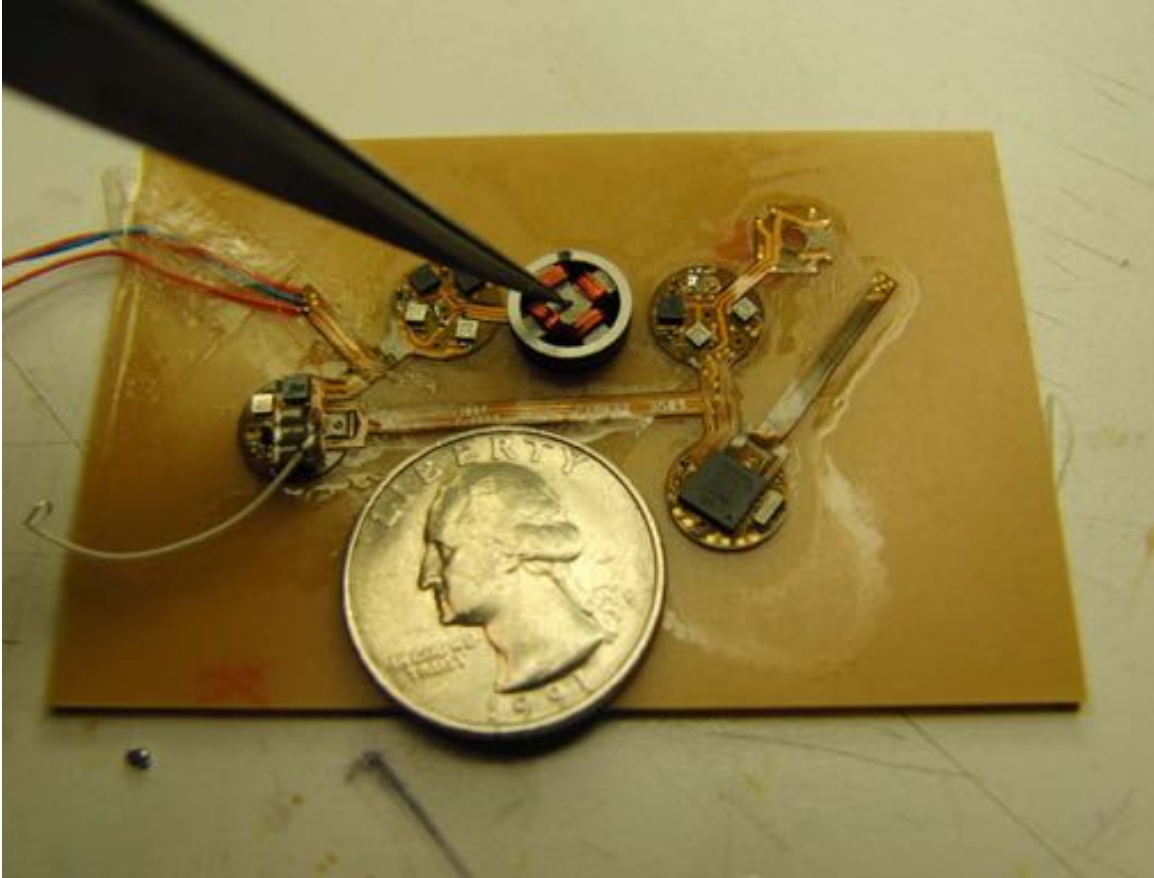
Figure 5-24: Complete friction-drive electropermanent stepper, shown with an early version of the Millibot flex circuit, which provides the drive pulses.
