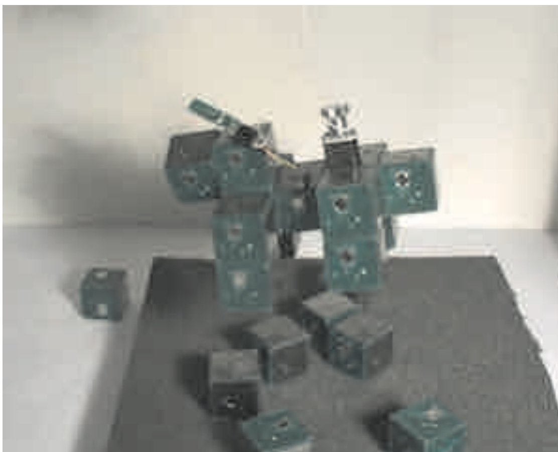
Figure 2-20: MICHE system forming a 15-module dog out of a 27-module block. The mechanically-switched permanent magnets release un-needed modules and they fall away. (Gilpin [35])
