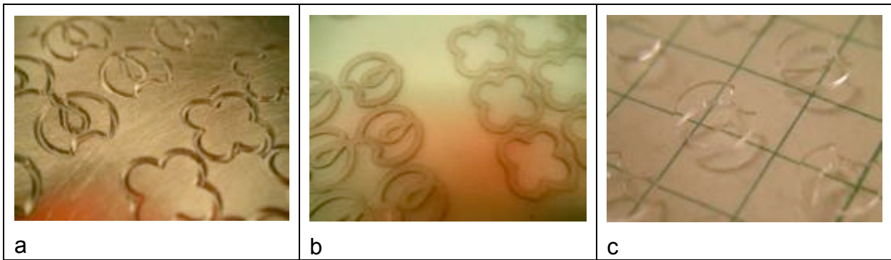
Figure 5-3 (a) Aluminum positive mold. (b) Polyurethane negative mold cast from (a). (c) PDMS SA components cast from (b) components were 4-8mm across.
