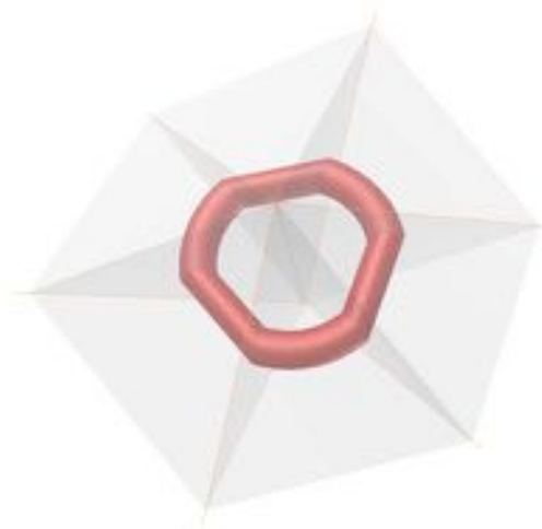
Figure 4-24. A rhombic hexahedron comprised of 6 right-angled tetrahedra, connected by a Hamiltonian loop that visits the centroid of all 6 sub-tetrahedra of the rhombic hexahedron.
