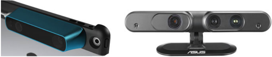
Fig. 2.2 Products based on the Primesense design: structure sensor by Occipital ( left ) and Asus X-tion Pro Live ( right )
