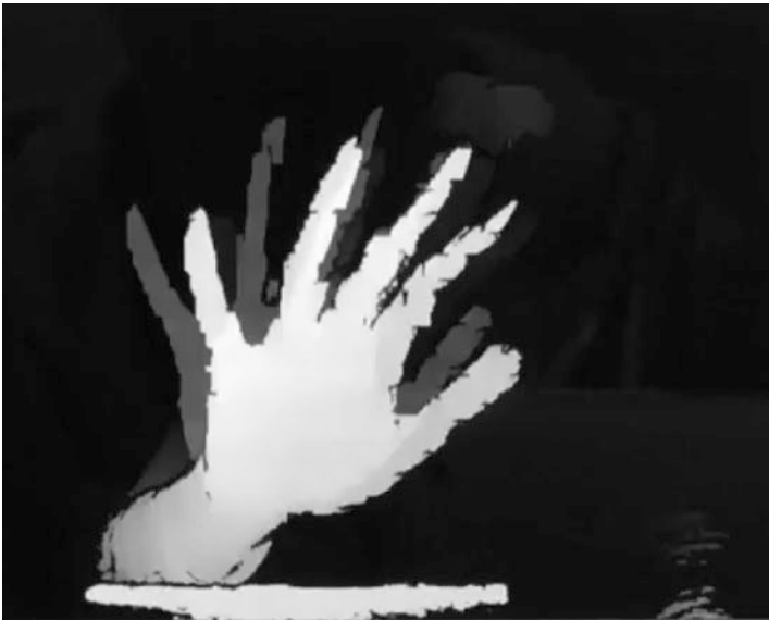
Fig. 2.16 Artifacts in the depth estimate of a moving hand acquired by the Intel RealSense F200 depth camera: the depth of the moving hand should only be the brightest silhouette, however a shadowed hand appears in the estimated depth map
