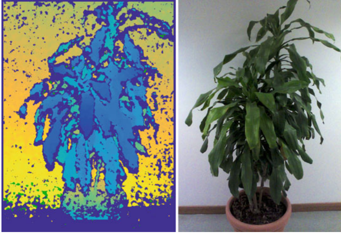
Fig. 2.33 The Intel RealSense R200 camera depth estimation process is based on spatial multiplexing, leading to coarse edges, as clearly shown from the depth map of the leaves of the framed plant
