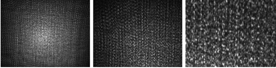
Fig. 2.31 Texture projected by the illuminator of the Intel RealSense R200 camera, framed at different zoom levels: ( left ) the full projected pattern; ( center ) a pattern zoom; ( right ) a macro acquisition
