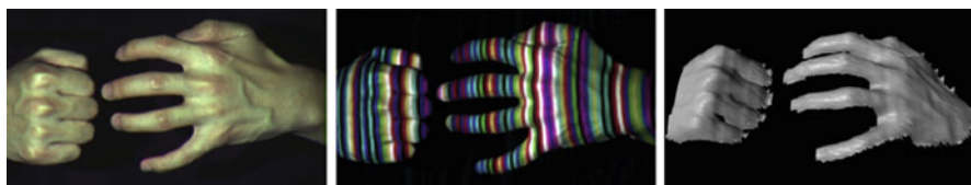
Fig. 2.9 Example of pattern projected by the illuminator of Zhang et al. ( center ) on a scene characterized by two hands ( left ), and the relative depth estimate ( right ). Courtesy of the authors of [21]
