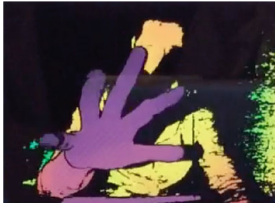
Fig. 2.27 Example of pixel-wise independent depth measurements obtained by the Intel RealSense F200 depth camera. The edges of the framed hand are pixel-precise and do not present edge jaggedness typical of spatial multiplexing techniques
